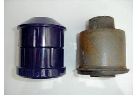
and inner metal tubes and for cracks appearing in the rubber – and not necessarily only at MOT time. Both symptoms will allow excessive flex and torsion beam movement, leading to vague and unpredictable handling or potentially erratic behaviour.
