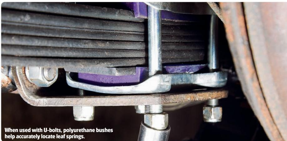
When used with U-bolts, polyurethane bushes help accurately locate leaf springs.
